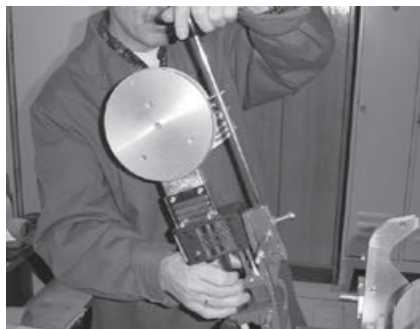
Fig. 1 Set the heat reflector in the holder
