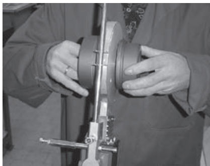
Fig. 2 Place the socket and the mandrel on the heat reflector
