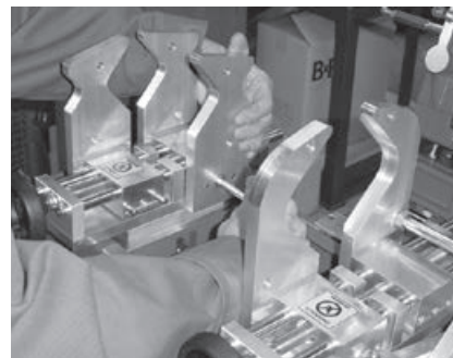
Fig. 3 Mount the prism clamping jaws
