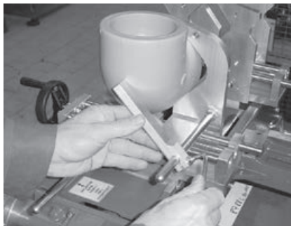
Fig. 7 Adjust the stop to hold the fittings
